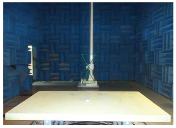
9.2. Photos of Radiated Measurement at Semi-Anechoic Chamber (Above 1GHz)
