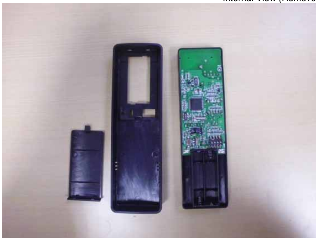
Photo 4 Internal View (Removed Cover)
