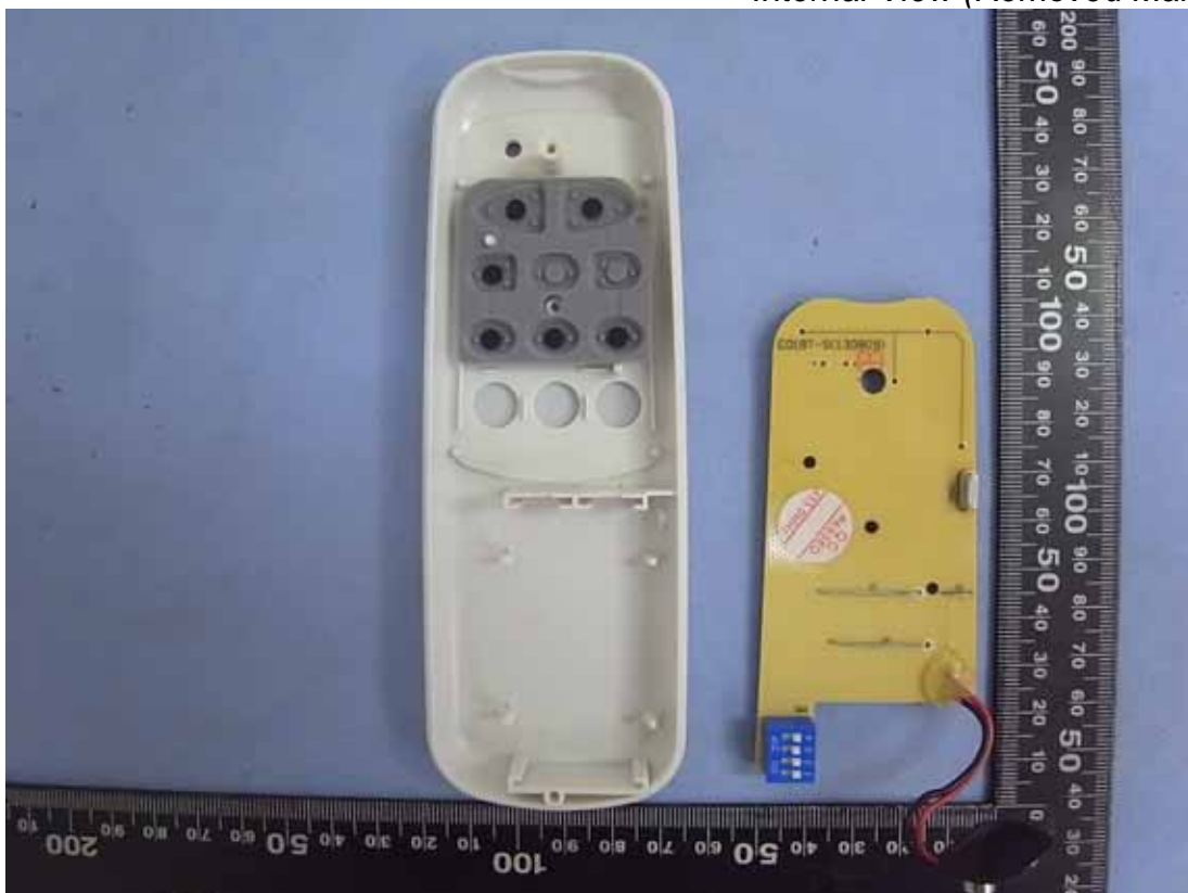
Photo 4 Internal View (Removed Main Board)
