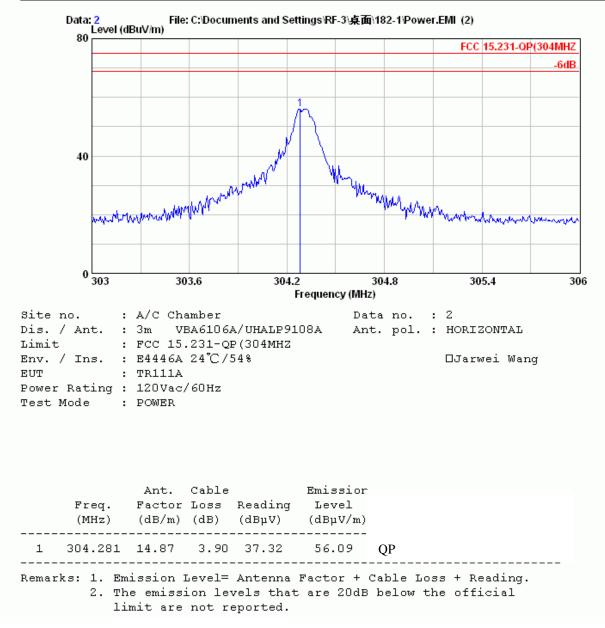
Horizontal is the strongest polarization and QP value has complied with limit, so vertical won't be listed in test report.
