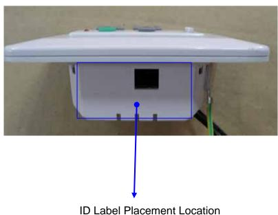
Label Placement Location (Side View of EUT)
