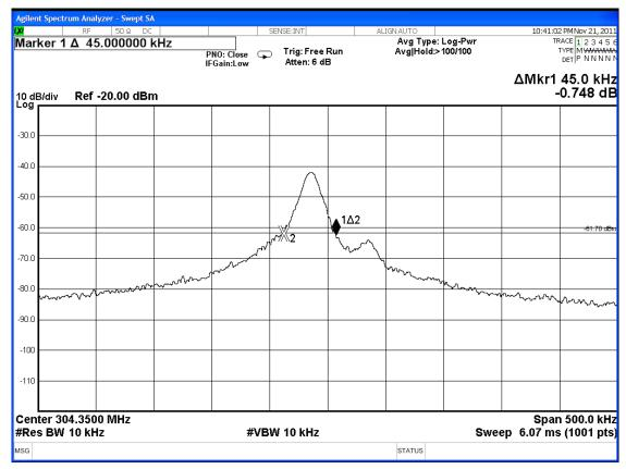
Note: "\$\times" The line is 20dB from the modulated carrier.
