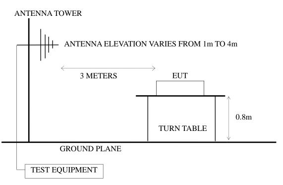
3.2.2. Semi-Anechoic Chamber (3m) Setup Diagram for 30-1000MHz
