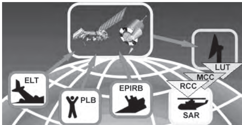
Figure 4 – Cospas Sarsat System Concept
