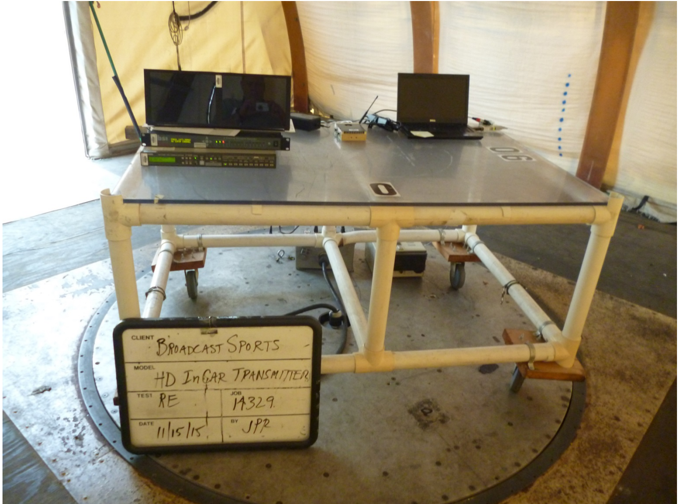
Photograph 1: Radiated Emission Test Configuration, Front
