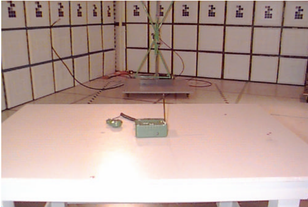
Maximized Radiated Emission Test Set-up – Front View
