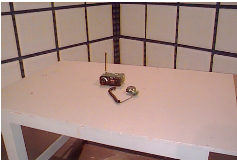
Maximized Radiated Emission Test Set-up – Front View
