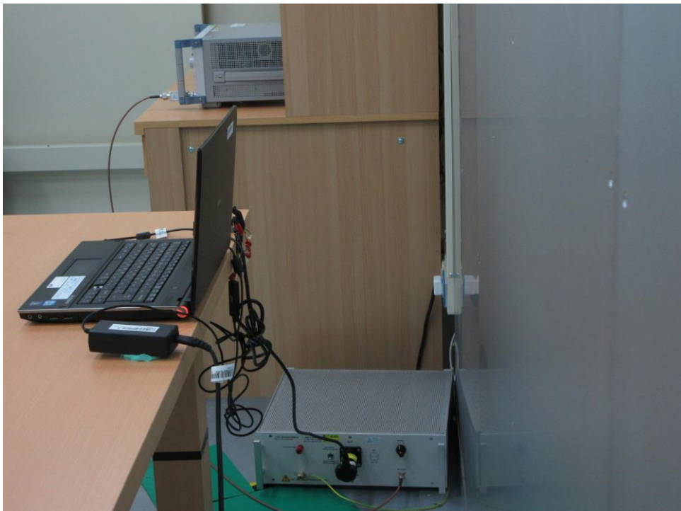
Photograph 8: Set-up for AC Mains (Back View)
