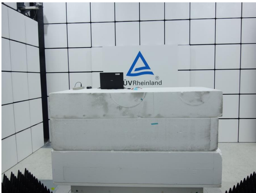
Photograph 2: Set-up for Spurious Emissions (Front View 2)
