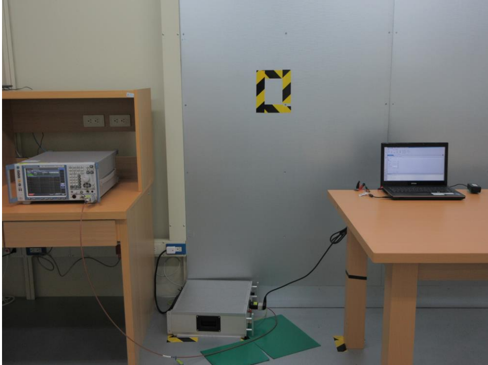
Photograph 7: Set-up for AC Mains (Front View)
