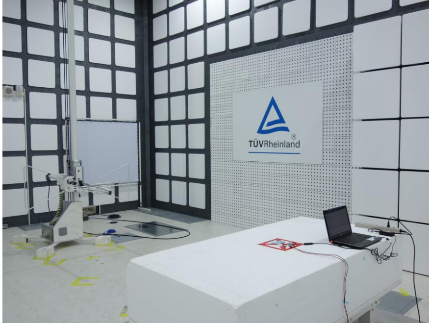
Photograph 3: Set-up for Spurious Emissions (Back View 1)
