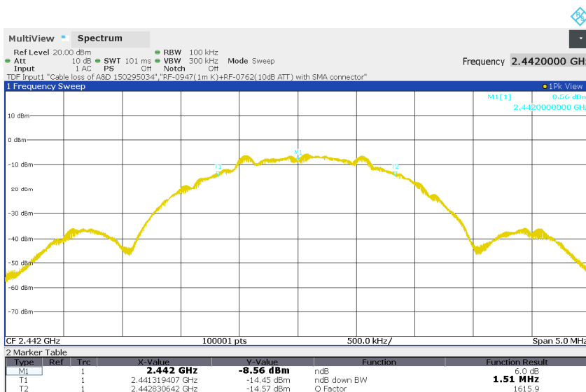
Figure 6: 6dB Bandwidth, BLE, Mode M (2442MHz), 2Mbps
