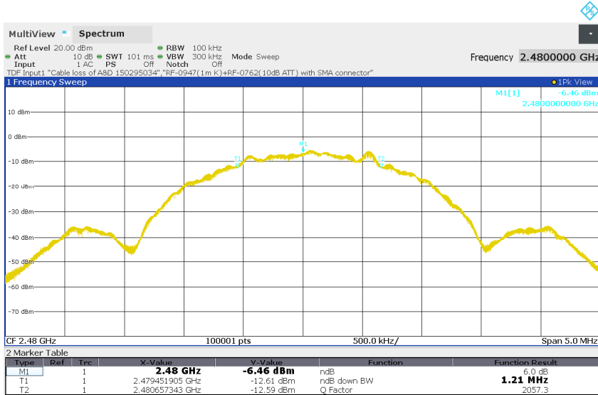
Figure 7: 6dB Bandwidth, BLE, Mode H (2480MHz), 2Mbps
