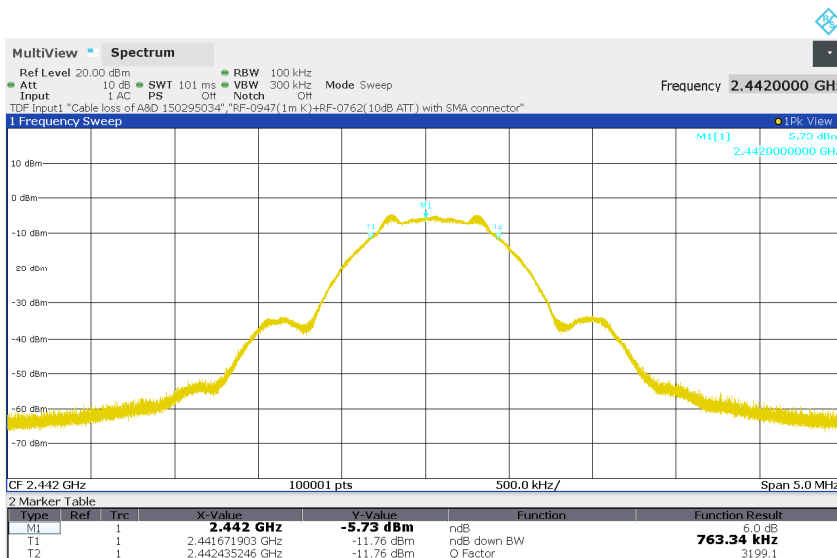
Figure 3: 6dB Bandwidth, BLE, Mode M (2442MHz), 1Mbps
