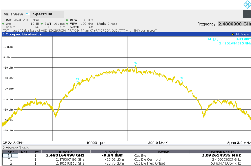
Figure 13: 99% Bandwidth, BLE, Mode H (2480MHz), 2Mbps
