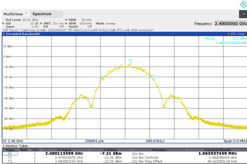
Figure 10: 99% Bandwidth, BLE, Mode H (2480MHz), 1Mbps
