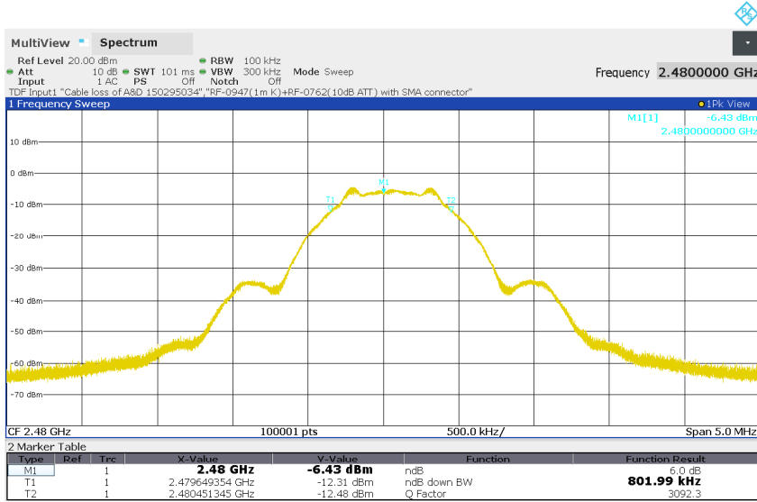
Figure 4: 6dB Bandwidth, BLE, Mode H (2480MHz), 1Mbps
