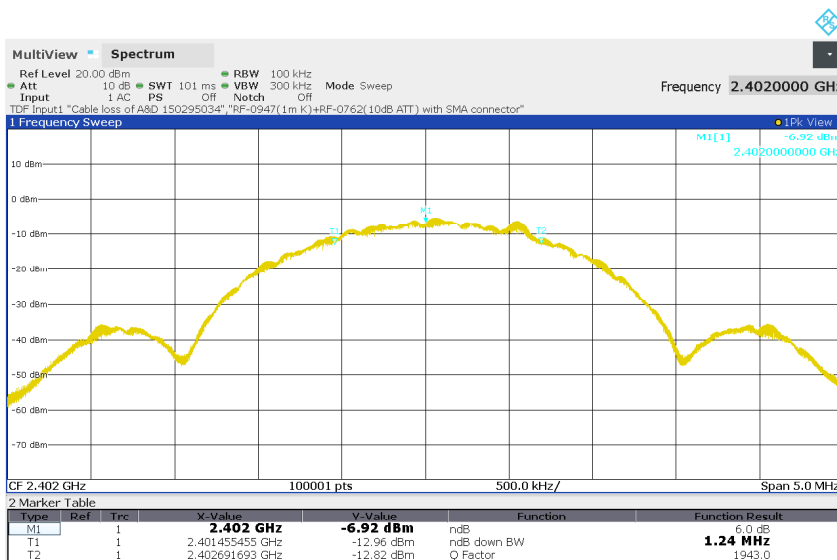
Figure 5: 6dB Bandwidth, BLE, Mode L (2402MHz), 2Mbps
