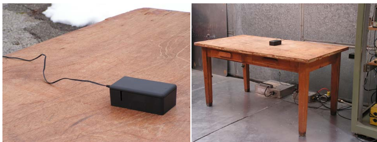
Photograph 6.6. Close-up of DUT on OATS + Conducted Emissions Setup
