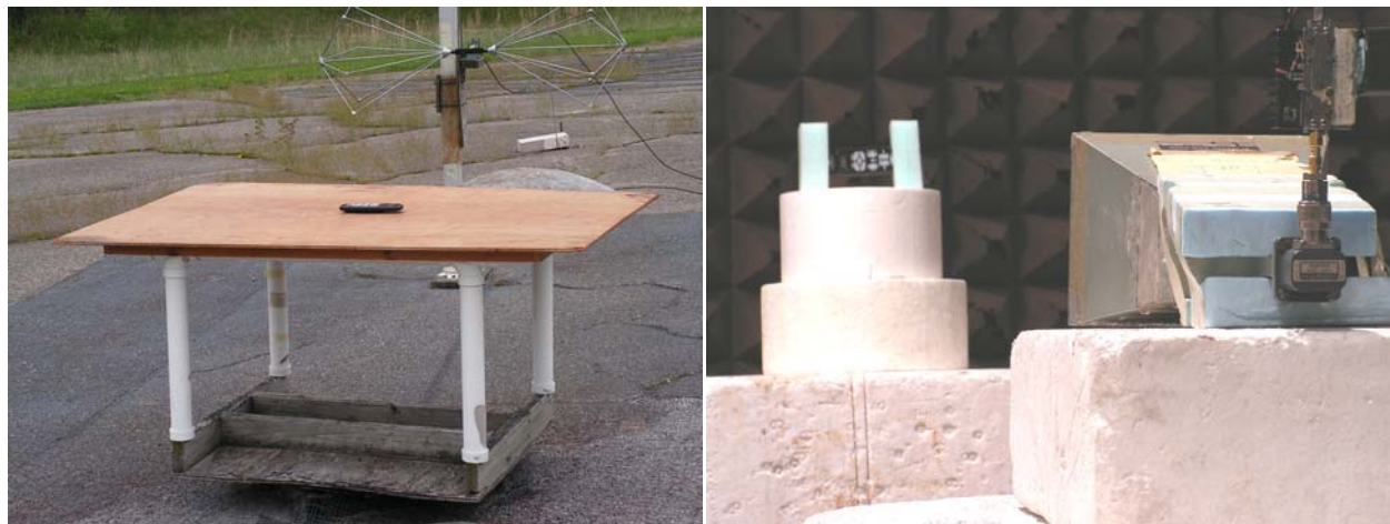
Photograph 6.5. DUT on OATS + Indoor Setup (one of three axes tested)
