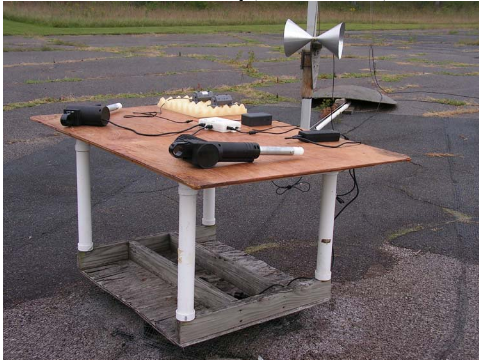
Test Setup (Radiated Emissions) – one of three axes tested
