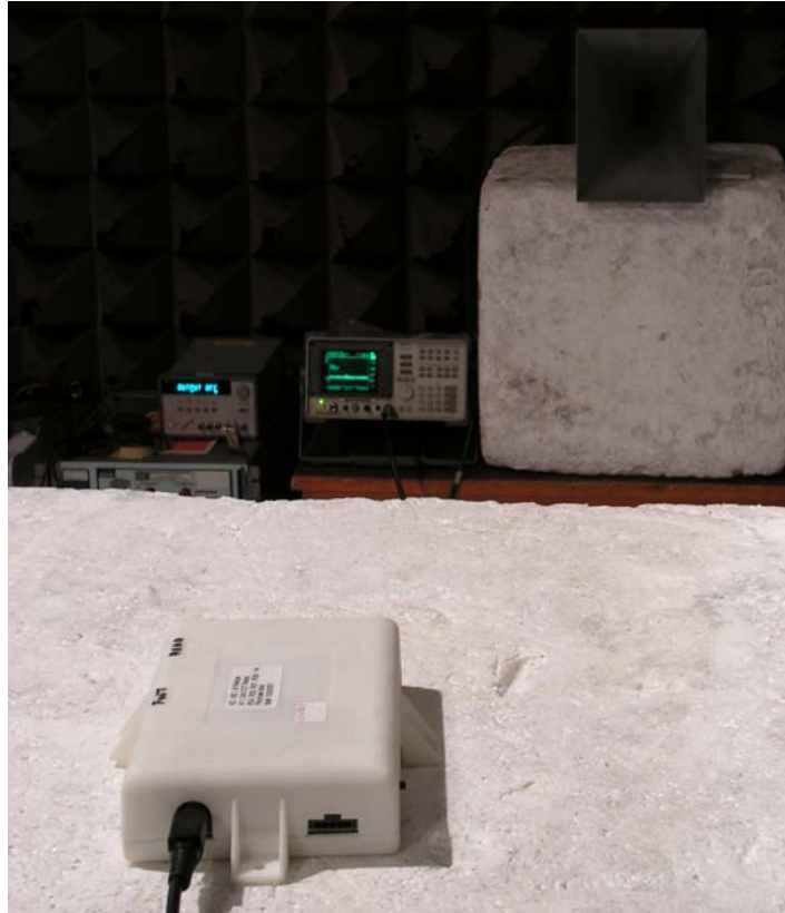
Test Setup (Radiated Emissions) – one of three axes tested
