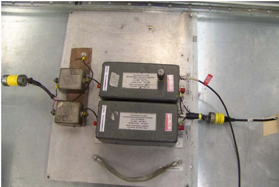
Conducted Emissions, Test Setup, Measurement Location, 115 VAC, 60 Hz Neutral into Steam Controller PC Board
