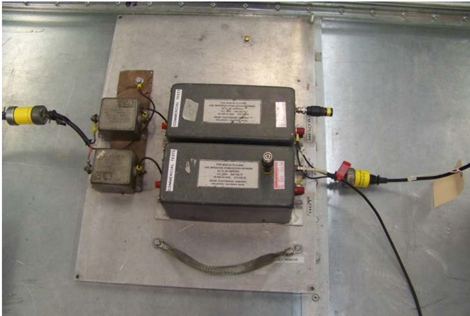
Conducted Emissions, Test Setup, Measurement Location, 115 VAC, 60 Hz Hot into Steam Controller PC Board
