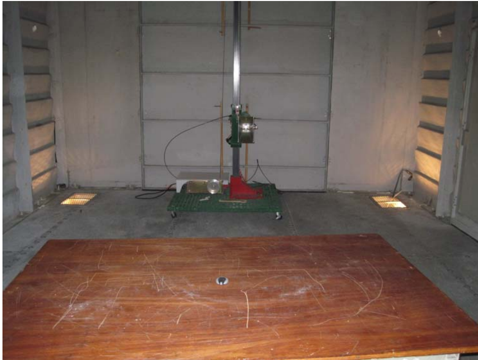
Receiver, Double Ridged Guide Antenna, Horizontal Polarity, Test Distance
