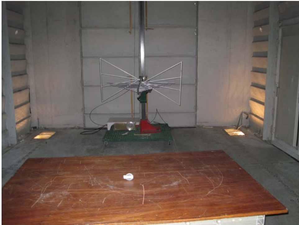
Receiver, Biconilog Antenna, Horizontal Polarity, Test Distance
