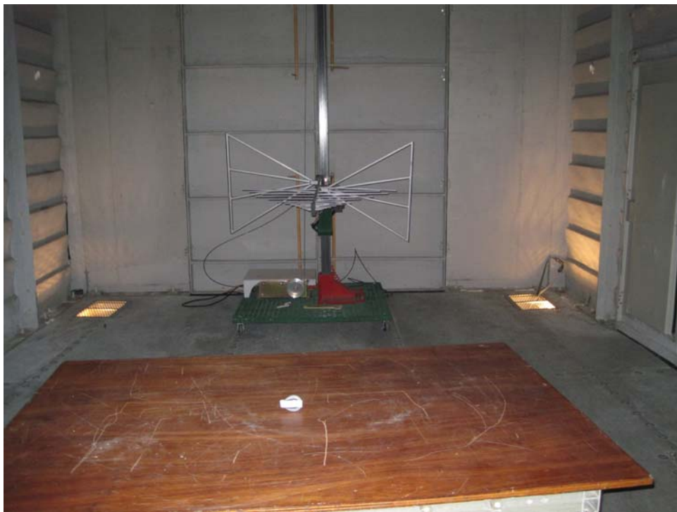
Transmitter, Biconilog Antenna, Horizontal Polarity, Test Distance
