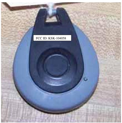
The device is too small for the FCC statement to appear on the device, therefore the FCC ID will be embossed on the back of the Key Fob and the warning statement shall be included in the User's Manual.
