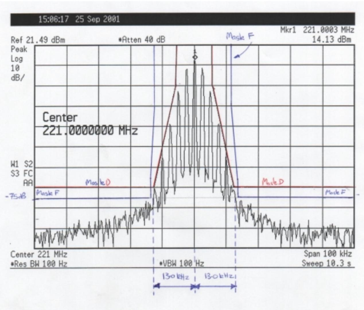
I trust that this shows that this transmitter meets the requirements of Section 90.733(e).
