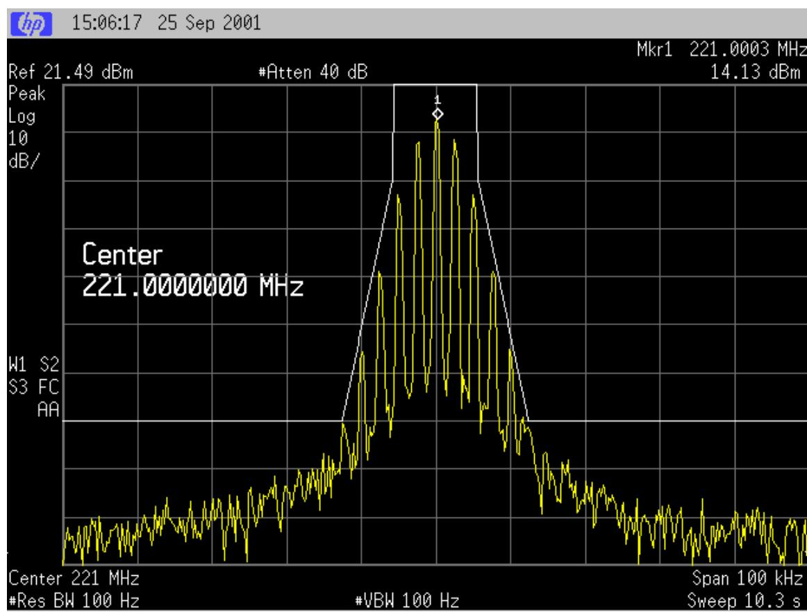
Emission mask F has been applied at the outermost edges of the contiguous channels.
