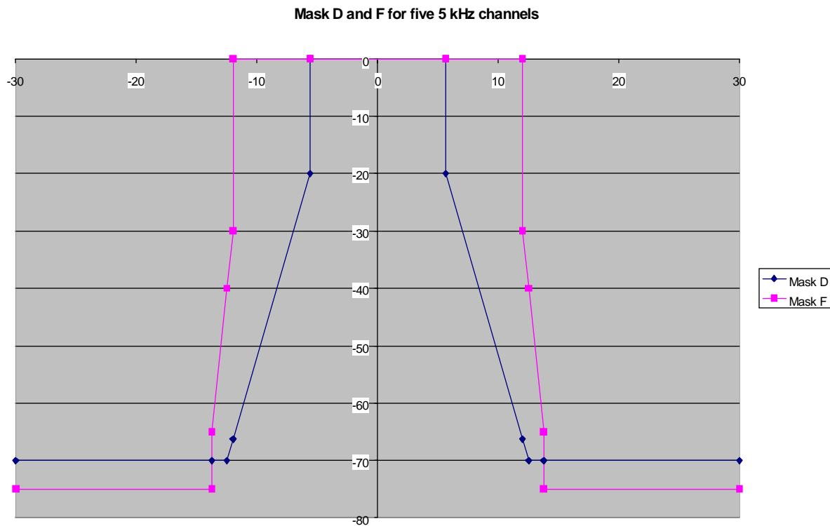
From this graph it can be seen that this transmitter would meet the requirements of emission mask F as per section 90.210(f) when five 5 kHz channels are utilised.
