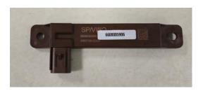
Antenna transmission frequency: 125kHz
