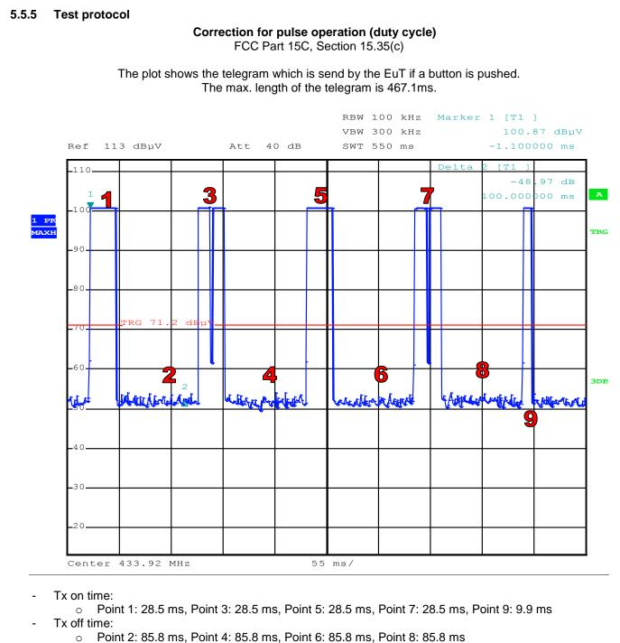
$\Rightarrow$  \* max. Tx on time within a 100 ms time period is 28.5 ms (Marker 1 and Delta 2)
