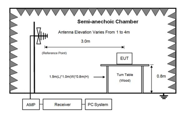
Semi-Anechoic 3m Chamber ANTENNA ELEVATION VARIES FROM 1 TO 4 METER 3m (Reference Point) 1.5m(L)\*1.0m(W)\*1.5m(H) **EUT TURN TABLE ABSORBER** (FIBRE GLASS) AMP PC System Spectrum Receiver
