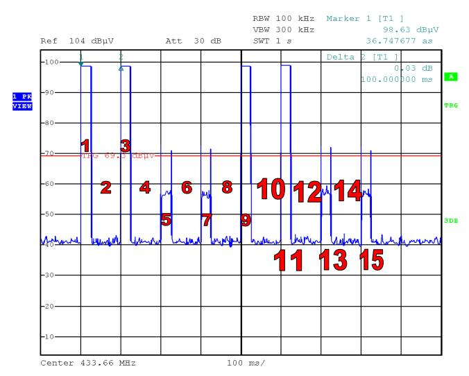
Tx on time: 24.0 ms at following points: 1, 3, 5, 7, 9, 11, 13, 15 Tx off time: 76.0 ms at following points: 2, 4, 6, 8, 10, 12, 14
