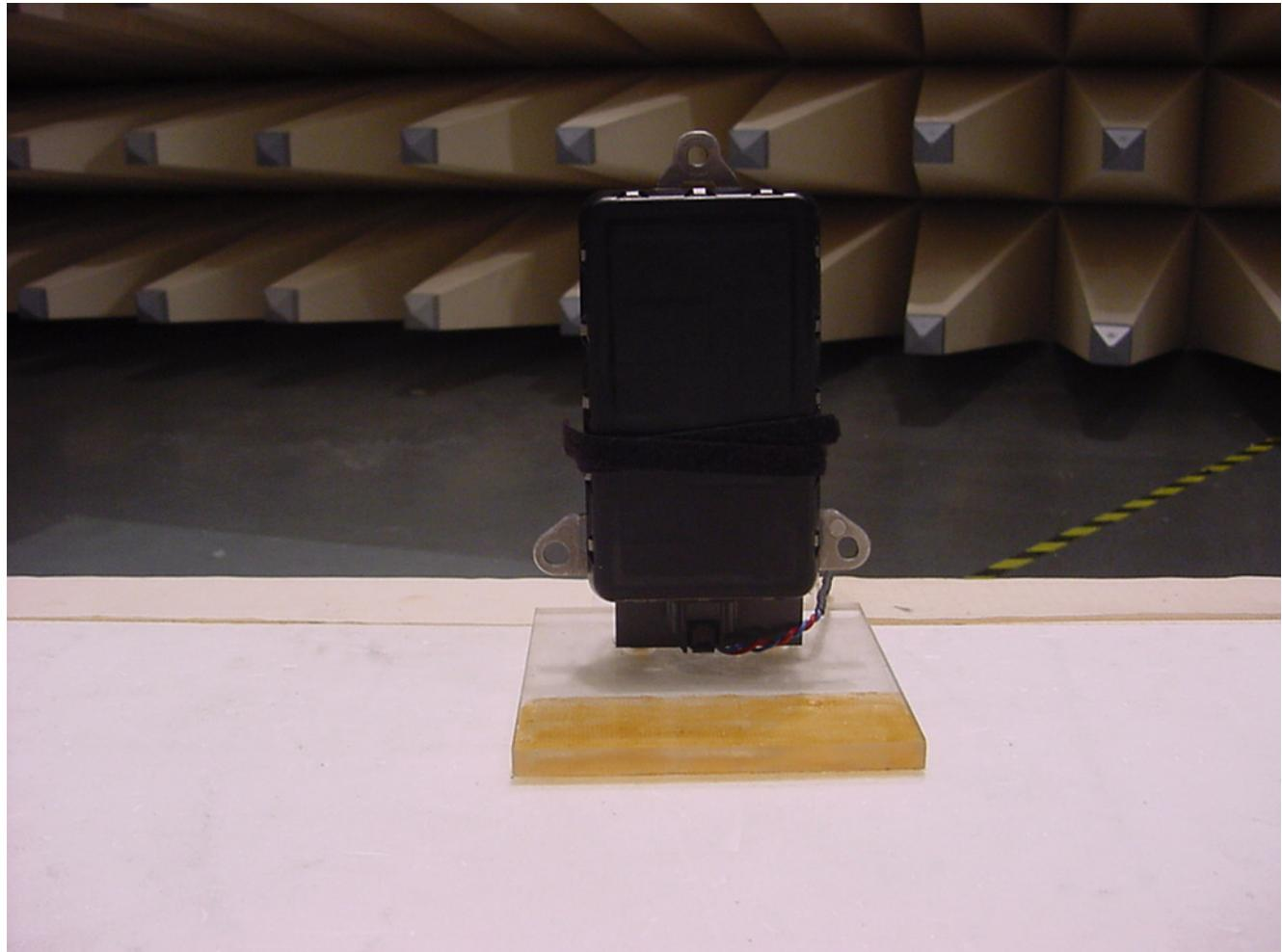
Radiated emissions measurement above 1.0 GHz
