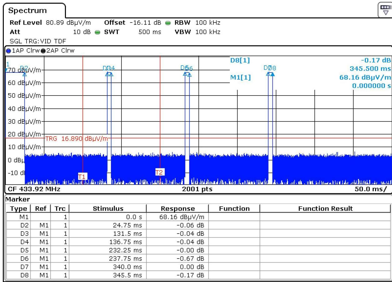
The Pulse train consists: one single pulse of 24.75 ms
