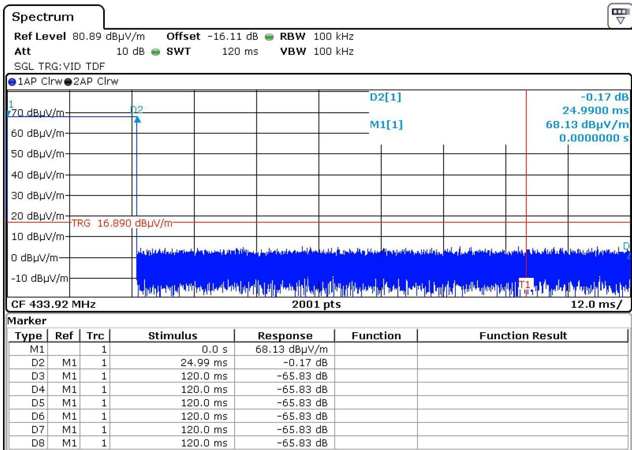
The measured worst case duration for a single pulse transmission in any 100ms time window is:
