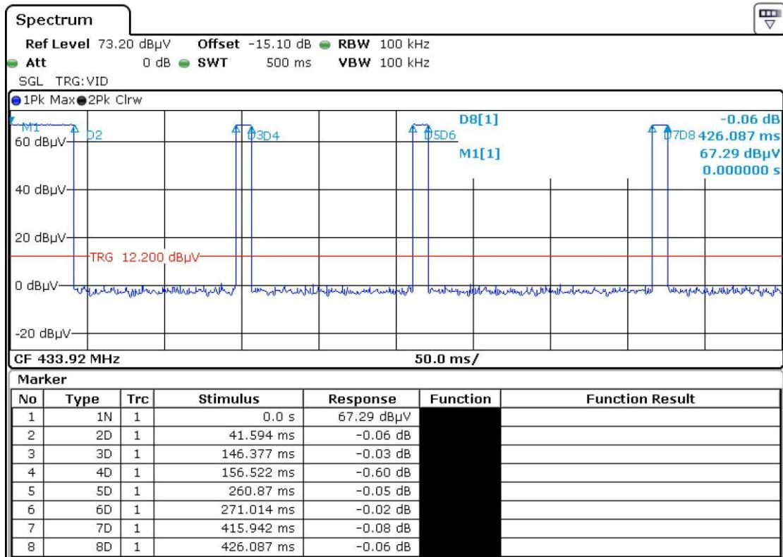
The Pulse train consists: one single pulse of 41.594 ms
