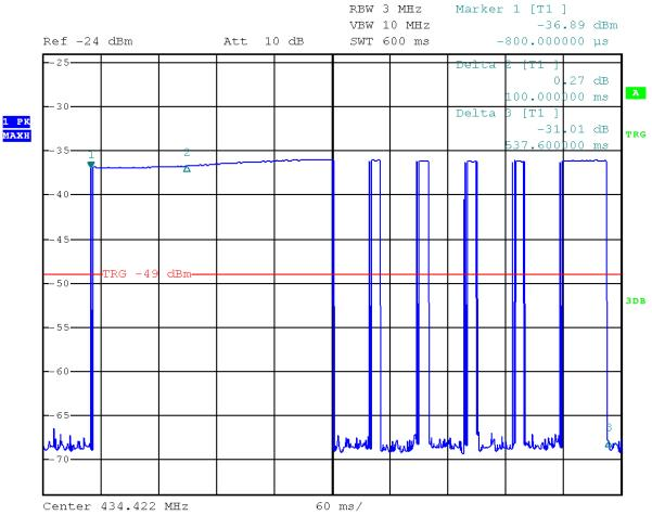
⇒ \* max. Tx on time within a 100 ms time period is 100 ms (Marker 1 and Delta 2)
