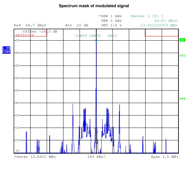
The values of the plot are extrapolated to a measurement distance of 3 m. (Calculated limit @ 3m: 124 dB $\mu$ V/m)
