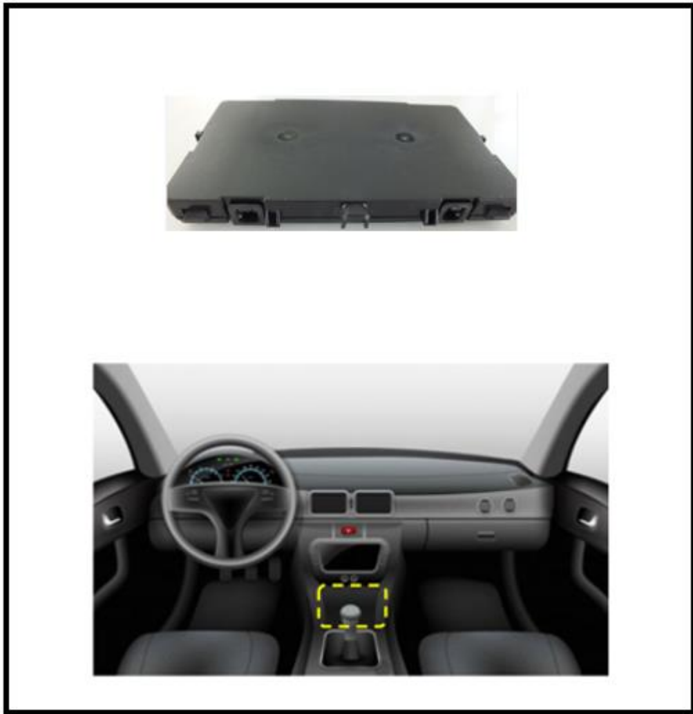
Fig. 1: NFC 3.0 module and its implementation inside the vehicle
