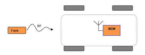
To lock and unlock the vehicle at distance a function is implemented in the system. The FOBIK transmit to the receiver an order. That it transmits on the CAN bus allows to achieve function  $\rightarrow$  No LF transmission
