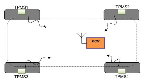
To control the pressure of vehicles wheels, the pressure captor (certificate done) transmit information to the BCM in RF. The BCM decode the signal (with RF Receiver) and transmit data on CSPI bus  $\rightarrow$  No LF transmission
