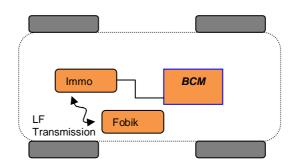
When the battery of Fobik is totally discharged, the BCM contains a function which pilots the antenna Room's 1. This antenna allows communicating at short distance with LF stage present on Fobik and to supply by field the Fobik to create a Carrier Wave signal. The LF coil which is used to communicate and authenticate Fobiks during Limp Home mode (125Khz).
