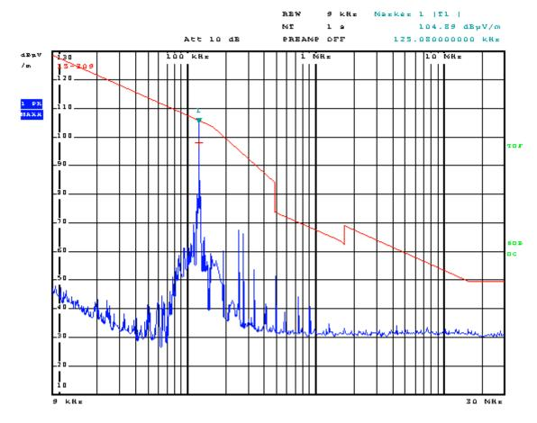
Picture 3: Radiated emission 9 kHz - 30 MHz @ 3m distance
