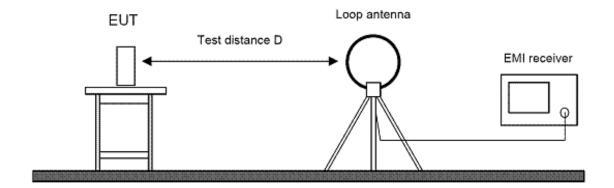
Picture 1: Test setup for radiated emission measurement (< 30 MHz)
