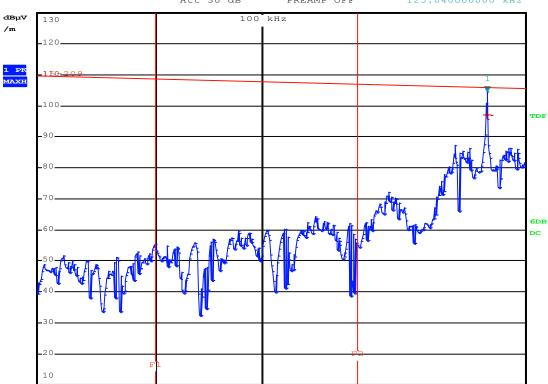
Picture 5: Restricted band of operation, AV @ 3m distance
