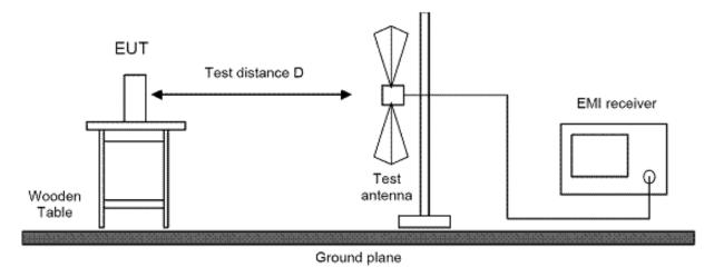
Picture 2: Test setup for radiated emission measurement (< 1 GHz)
