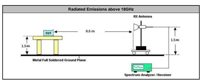
Note 1: Magnetic field tests shall be performed in the frequency range of 9 kHz to 30 MHz using a calibrated loop antenna. Electric field tests shall be performed in the frequency range of 30 MHz to 1000 MHz using a calibrated bi-log antenna and the frequency range of 1 GHz to 40 GHz using a calibrated horn antenna. Note 2: If test distance other than 3m is used, the used test distance will be recorded in test result.
