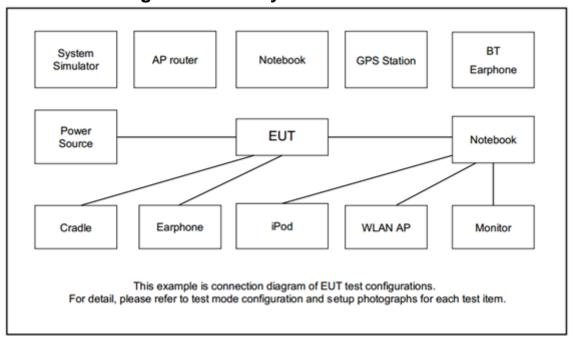
2.3. Support Unit used in test configuration and system
