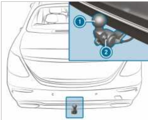
Trailer hitch (example with additional guide pins)
