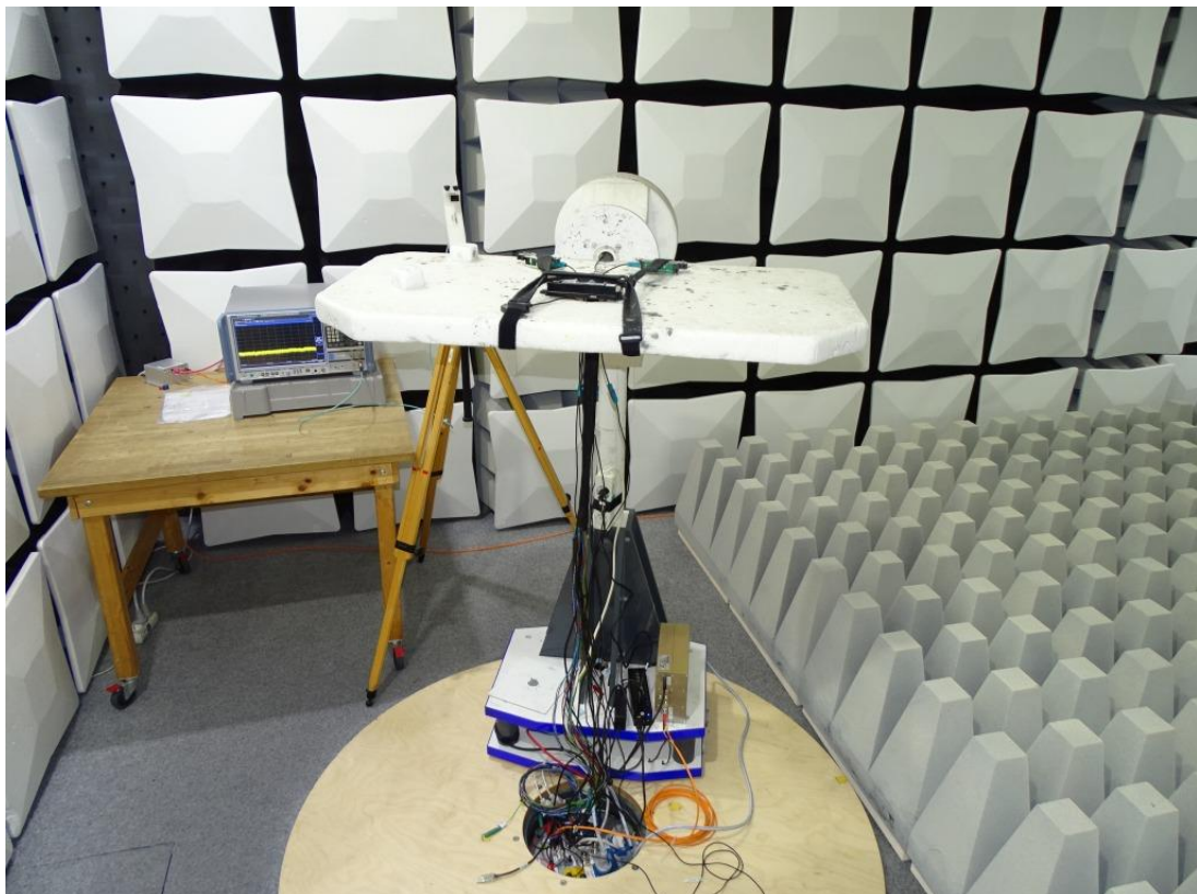
Photo 4: Test setup for radiated measurements above 26 GHz
