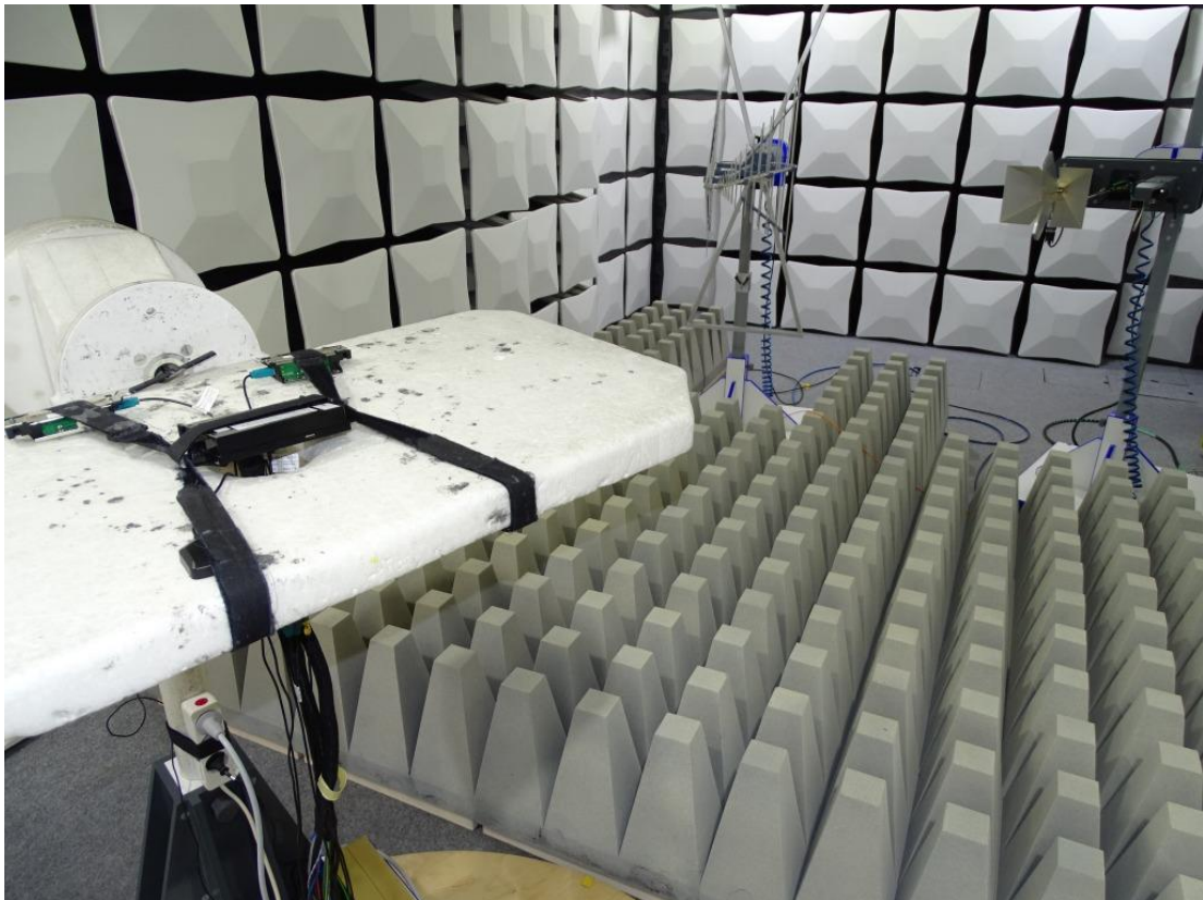
Photo 3: Test setup for radiated measurements above 1 GHz
