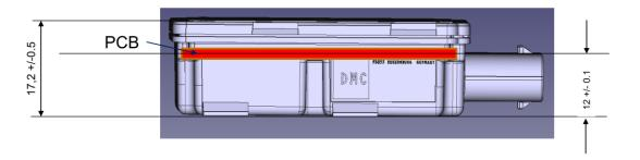
As shown on the drawing above, the inherent minimum separation distance between the radiating element(s) and any person is stated as being  $12 \pm 0.1$  mm.
