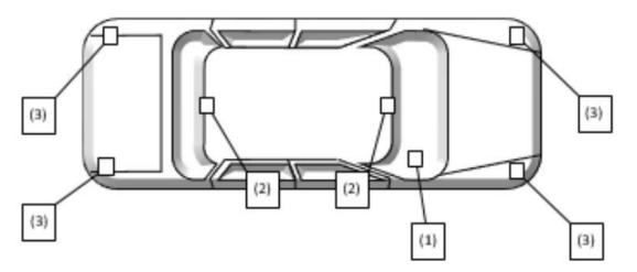
Two other devices are fitted in the positions indicated by (2). These devices are described in a corresponding filing for FCC ID: KR5FBD5. Each of these devices contains an UWB transmitter similar to the UWB transmitter as described in this filing and also contain 2 BLE transmitters.
