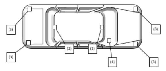
Four other devices are fitted in the positions indicated by (3). These devices are described in a corresponding filing for FCC ID: KR5FBD5S. Each of these devices contains an UWB transmitter similar to the UWB transmitter as described in this filing, except that these devices, as described in a corresponding filing for FCC ID: KR5FBD5S, do not contain a BLE transmitter.
