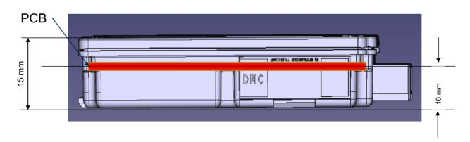
As shown on the drawing above, the inherent minimum separation distance between the radiating element(s) and any person is stated as being 10 mm.
