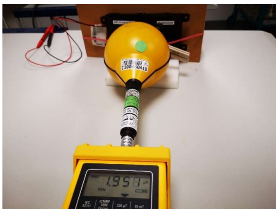
Photograph 32: Measurements in the shielded room, 7.3 cm distance between measurement probe and EUT, Position 5, H-Field, 5% charging level
