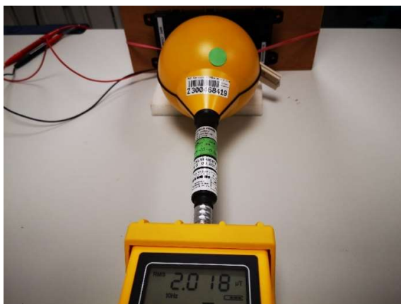
Photograph 15: Measurements in the shielded room, 7.3 cm distance between measurement probe and EUT, Position 5, H-Field, 5% charging level
