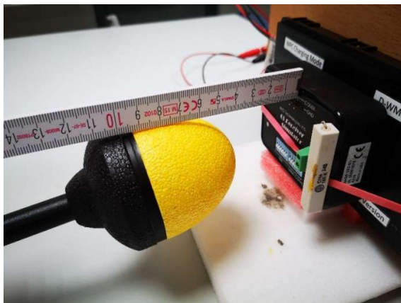
Photograph 23: Measurements in the shielded room, 7.3 cm distance between measurement probe and EUT, Position 5, E-Field, 50% charging level
