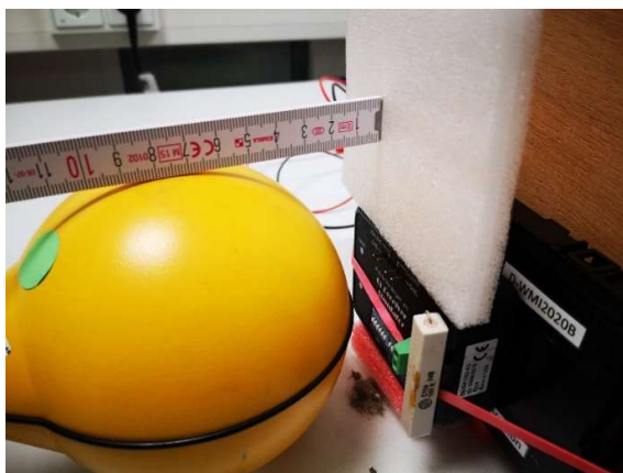
Photograph 29: Measurements in the shielded room, 7.3 cm distance between measurement probe and EUT, Position 5, H-Field, 50% charging level
