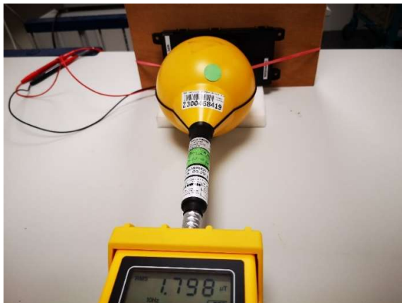
Photograph 11: Measurements in the shielded room, 7.3 cm distance between measurement probe and EUT, Position 5, H-Field, 90% charging level
