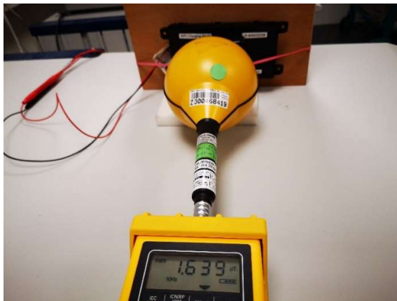
Photograph 28: Measurements in the shielded room, 7.3 cm distance between measurement probe and EUT, Position 5, H-Field, 90% charging level
