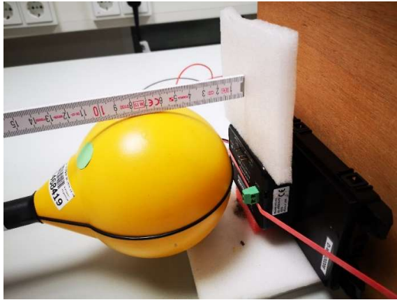
Photograph 10: Measurements in the shielded room, 7.3 cm distance between measurement probe and EUT, Position 5, H-Field
