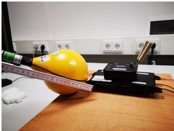
Photograph 34: Measurements in the shielded room, 6.2 cm distance between measurement probe and EUT, Position 4, H-Field, 5% charging level
