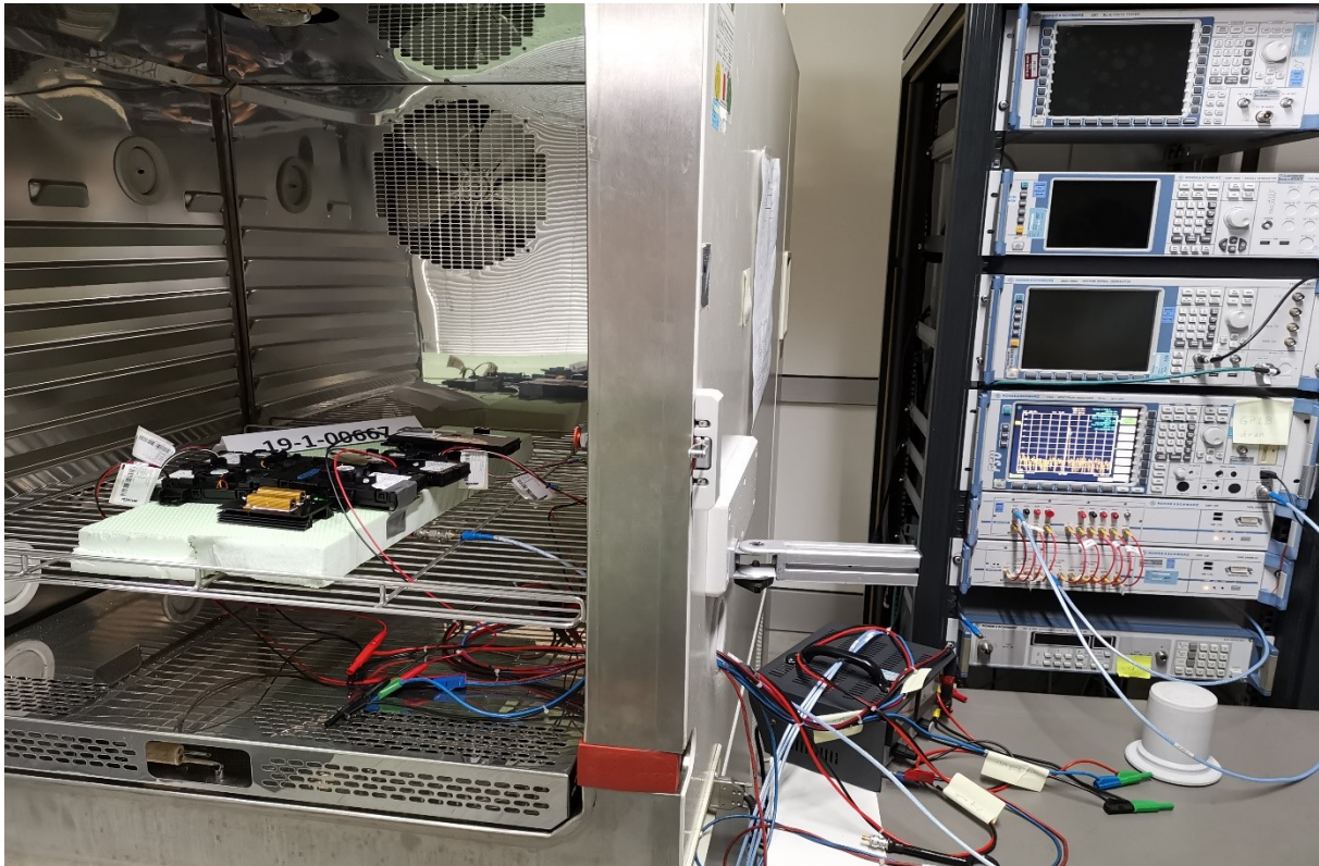
Photograph 1: EUT inside climate chamber- Overall View, set-up. 4 + 5, Op.1
