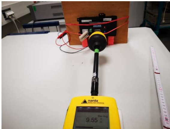
Photograph 9: Measurements in the shielded room, 9.7 cm distance between measurement probe and EUT, Position 5, E-Field, 5% charging level
