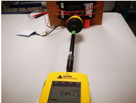
Photograph 38: Measurements in the shielded room, 9.7 cm distance between measurement probe and EUT, Position 5, E-Field, 90% charging level
