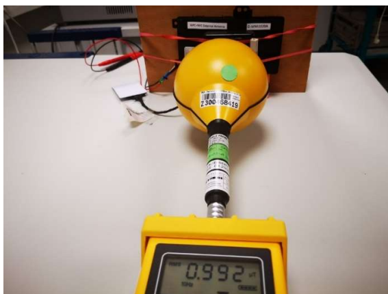
Photograph 29: Measurements in the shielded room, 9.7 cm distance between measurement probe and EUT, Position 5, H-Field, 50% charging level
