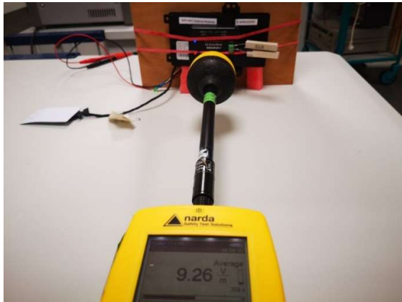
Photograph 25: Measurements in the shielded room, 9.7 cm distance between measurement probe and EUT, Position 5, E-Field, 5% charging level
