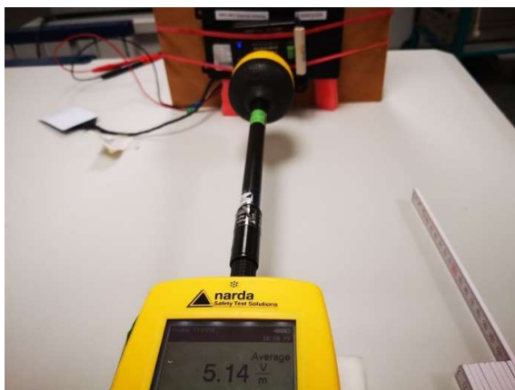
Photograph 23: Measurements in the shielded room, 9.7 cm distance between measurement probe and EUT, Position 5, E-Field, 50% charging level
