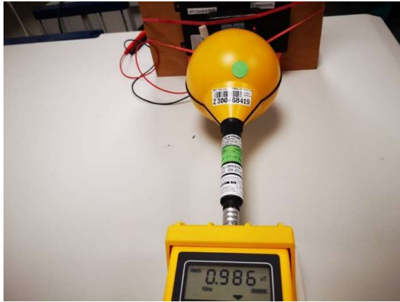
Photograph 13: Measurements in the shielded room, 9.7 cm distance between measurement probe and EUT, Position 5, H-Field, 50% charging level
