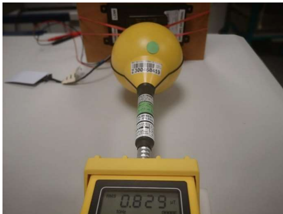
Photograph 44: Measurements in the shielded room, 9.7 cm distance between measurement probe and EUT, Position 5, H-Field, 90% charging level
