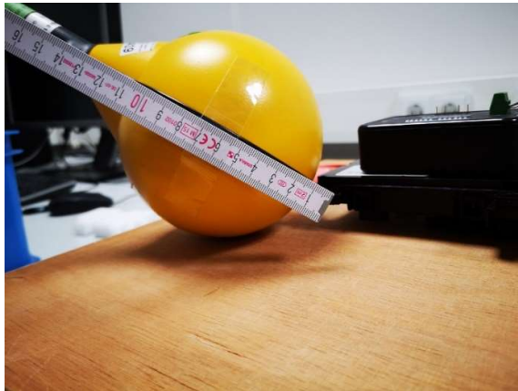
Photograph 17: Measurements in the shielded room, 6.2 cm distance between measurement probe and EUT, Position 4, H-Field, 5% charging level
