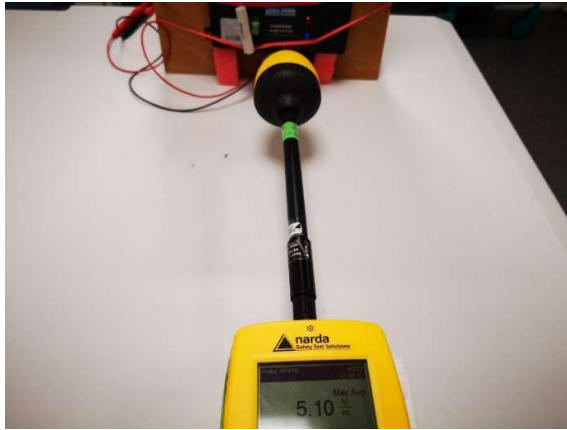
Photograph 7: Measurements in the shielded room, 9.7 cm distance between measurement probe and EUT, Position 5, E-Field, 5% charging level
