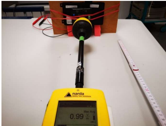
Photograph 5: Measurements in the shielded room, 9.7 cm distance between measurement probe and EUT, Position 5, E-Field, 90% charging level
