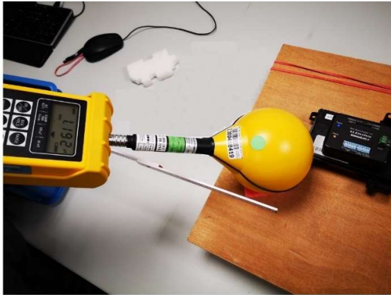
Photograph 16: Measurements in the shielded room, 6.2 cm distance between measurement probe and EUT, Position 4, H-Field, 5% charging level
