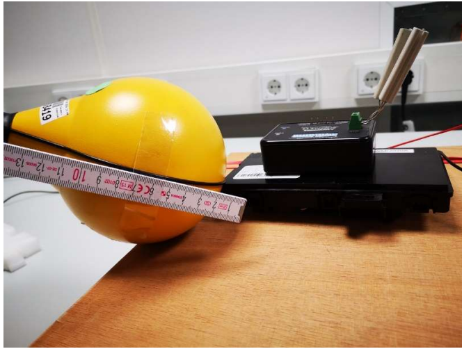
Photograph 33: Measurements in the shielded room, 6.2 cm distance between measurement probe and EUT, Position 4, H-Field, 5% charging level
