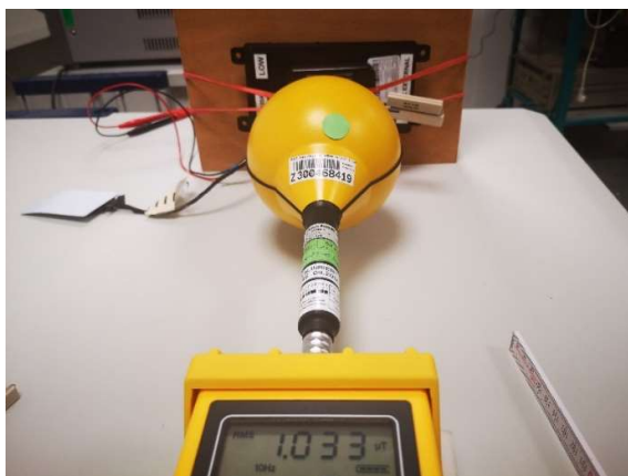
Photograph 48: Measurements in the shielded room, 9.7 cm distance between measurement probe and EUT, Position 5, H-Field, 5% charging level
