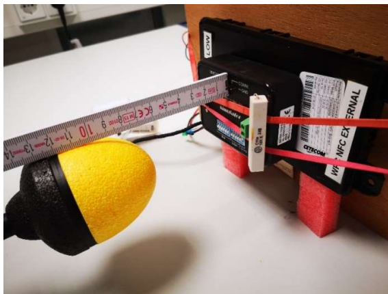
Photograph 39: Measurements in the shielded room, 9.7 cm distance between measurement probe and EUT, Position 5, E-Field, 50% charging level
