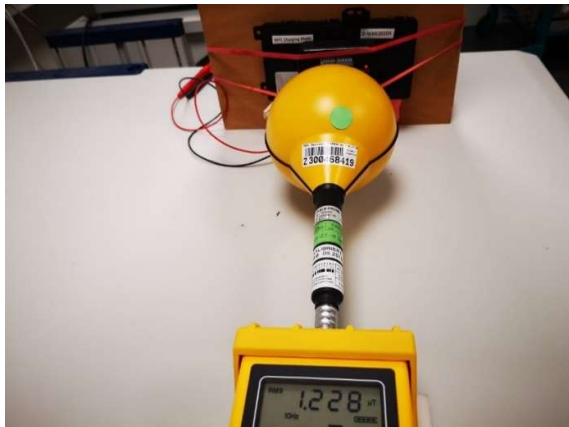
Photograph 15: Measurements in the shielded room, 9.7 cm distance between measurement probe and EUT, Position 5, H-Field, 5% charging level
