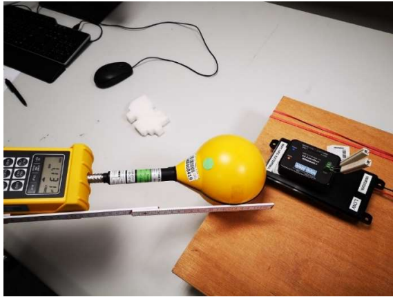
Photograph 49: Measurements in the shielded room, 6.2 cm distance between measurement probe and EUT, Position 4, H-Field, 5% charging level
