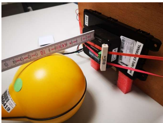
Photograph 45: Measurements in the shielded room, 9.7 cm distance between measurement probe and EUT, Position 5, H-Field, 50% charging level
