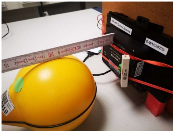
Photograph 28: Measurements in the shielded room, 9.7 cm distance between measurement probe and EUT, Position 5, H-Field, 50% charging level
