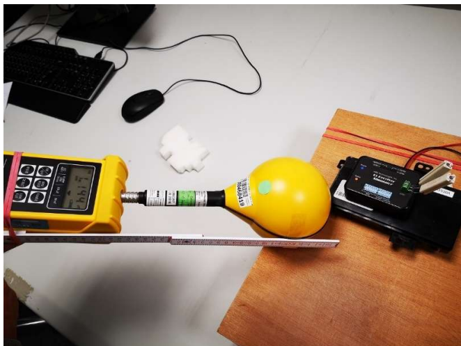
Photograph 32: Measurements in the shielded room, 6.2 cm distance between measurement probe and EUT, Position 4, H-Field, 5% charging level
