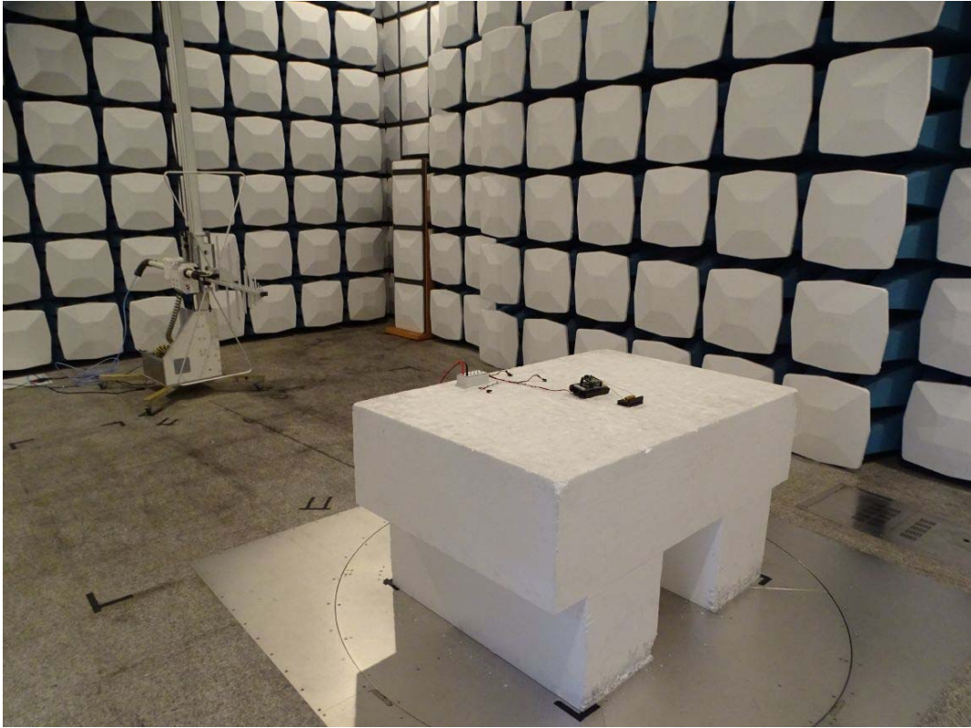
Back View of Radiated Test
