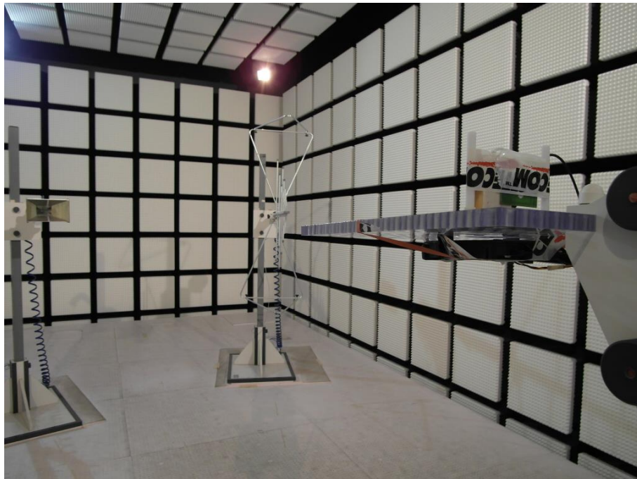
Photo 16 (RSE set-up with external antenna / Fully-anechoic chamber):
