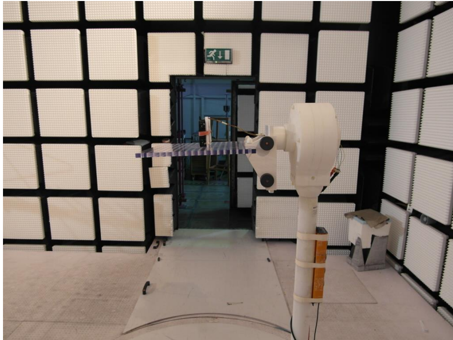
Photo 11 (RSE set-up with ID-card / Fully-anechoic chamber):
