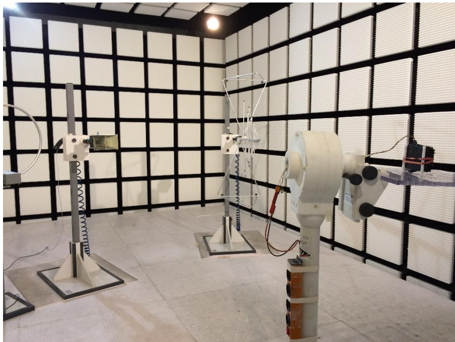
Photo 3 (RSE set-up / Fully-anechoic chamber):
