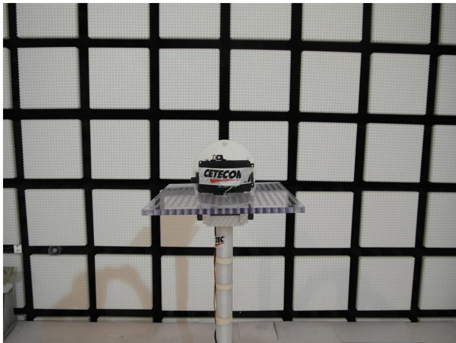
Photo 5 (RSE set-up with wireless charging unit / Fully-anechoic chamber):
