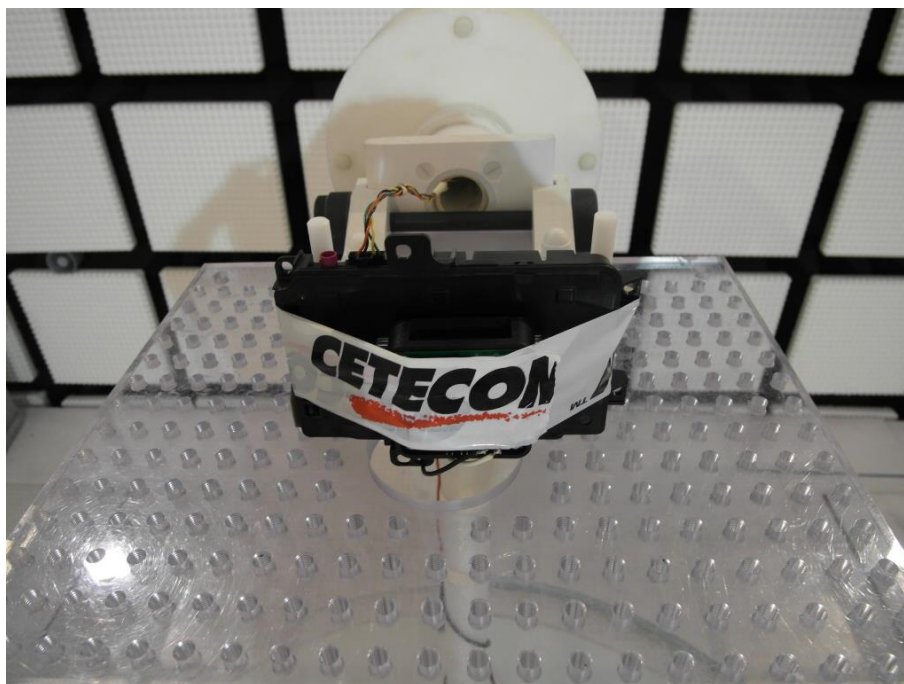
Photo 6 (RSE set-up with wireless charging unit / Fully-anechoic chamber):
