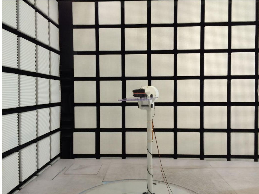
Photo 1 (RSE set-up / Fully-anechoic chamber):
