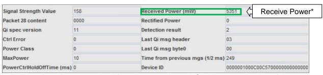
EUT interface: Data transmitted from the smartphone. \* Slightly overestimation of the Received Power (typically < 250mW)
