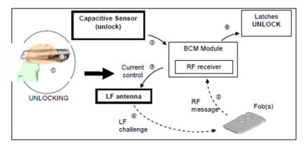
As the user's hand approaches the capacitive sensor UNLOCK detection area, sensor communicates detection to BCM Module. Then, the corresponding LF antenna on front side is driven by system to send LF challenge to fob(s) to perform the user's identification process.
