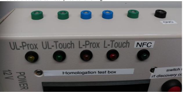
For each lead an output is available and can be connected directly to any recorder (oscilloscope,...). High level means no detection, low level means detection.
