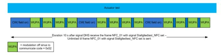
REQA is replaced by WUPA to ensure several communication possible whereas field is kept on.
