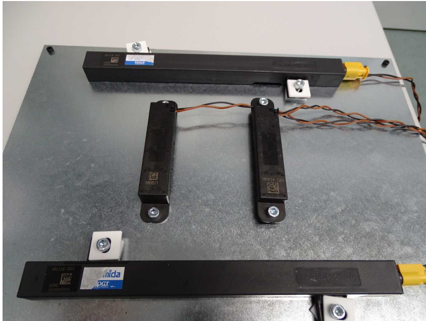
Photo 7: The four external antennas
