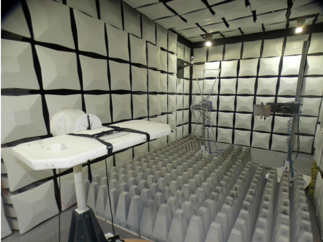
Photo 3: Test setup for radiated measurements above 1 GHz
