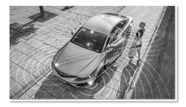
The Mercedes-Benz CMBTRX1 is a UWB (Ultra Wide Band) and BLE (Bluetooth® Low Energy) transceiver module for car access and user localization purposes. Two CMBTRX1 are mounted in the headliner of the car and four in the front and rear bumpers. They are all connected to a central control unit via CAN interface.
