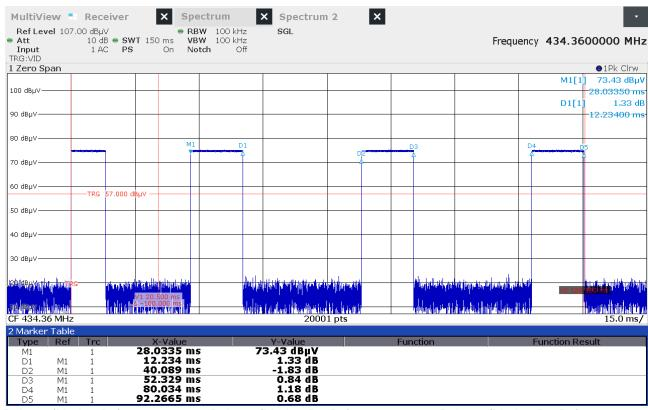
Pulse 1 (Marker D1): 12.234 ms Pulse 2 (Marker D3-D2): 12.240 ms Pulse 3 (Marker D5-D4): 12.232 ms
