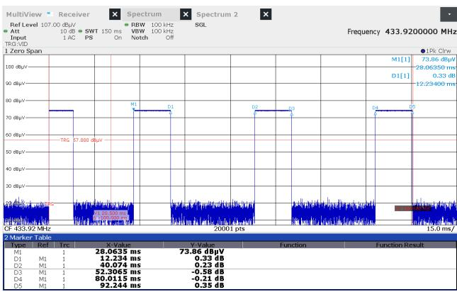
Pulse 1 (Marker D1): 12.234 ms Pulse 2 (Marker D3-D2): 12.233 ms Pulse 3 (Marker D5-D4): 12.233 ms **Max. total on time within 100 ms = 36.700 ms**
