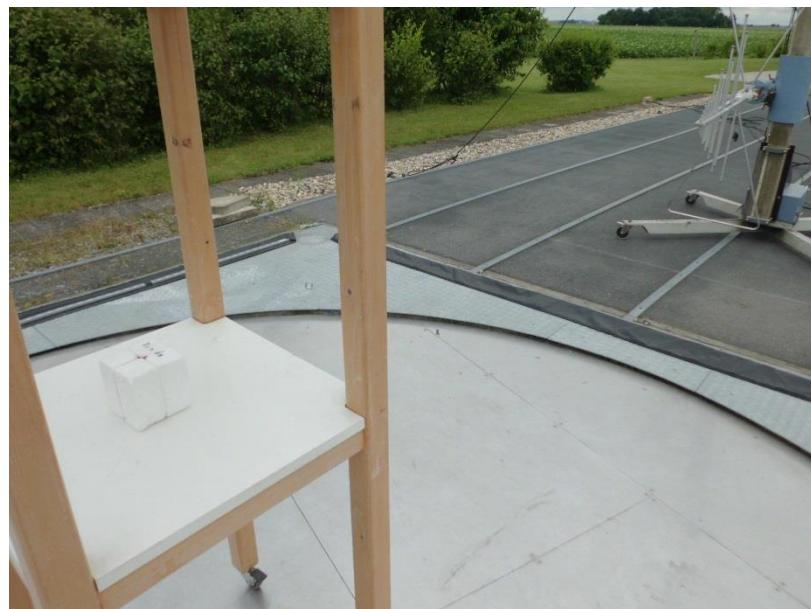
Out of band emissions 9 kHz – 30 MHz
