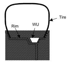
It is made of a PCB that supports the electronic hardware encapsulated inside a box and polyurethane foam. It is self-powered by a battery and includes all systems for measurements (pressure, temperature, centrifugal acceleration, and battery status), RF emission and LF reception.
