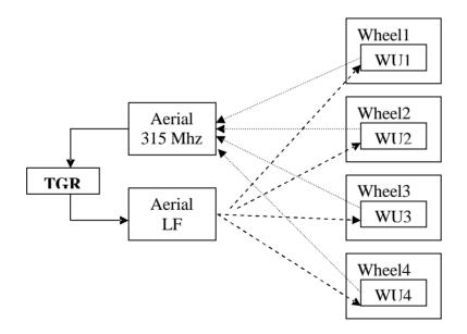
LF triggering is made by some specific LF drivers and antennas. RF reception is made by one antenna linked to the TGR. LF triggering is only used in case of axle localization.
